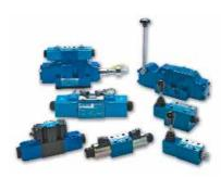
DG valves mount on industry standard surfaces and provide 3 or 4-way control in a broad range of applications, industrial and mobile. Their primary function is to direct fluid flow to a cylinder or to control the direction of rotation of a hydraulic motor. These valves can be actuated by solenoid, hydraulic or pneumatic pilot, lever, or mechanically.
